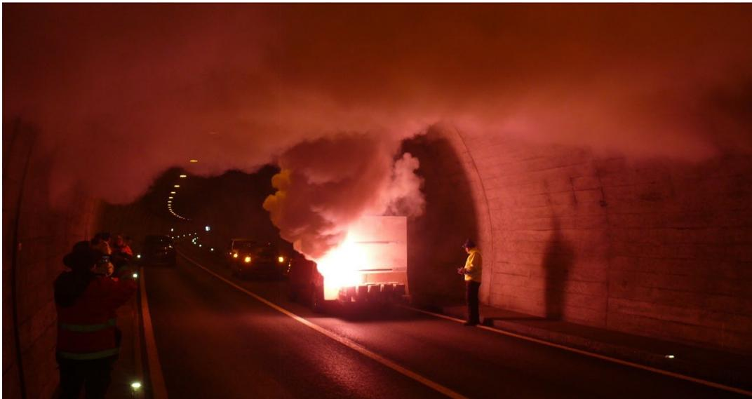
Figure 15: Hot smoke Test in a Road Tunnel
