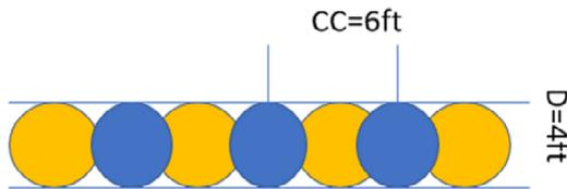
Figure 6 Proposed Secant Pile Configuration
