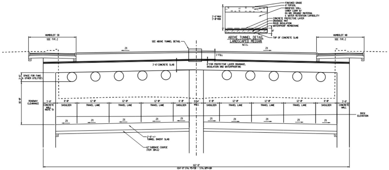
Figure 3 Tunnel Roadway Cross Section
