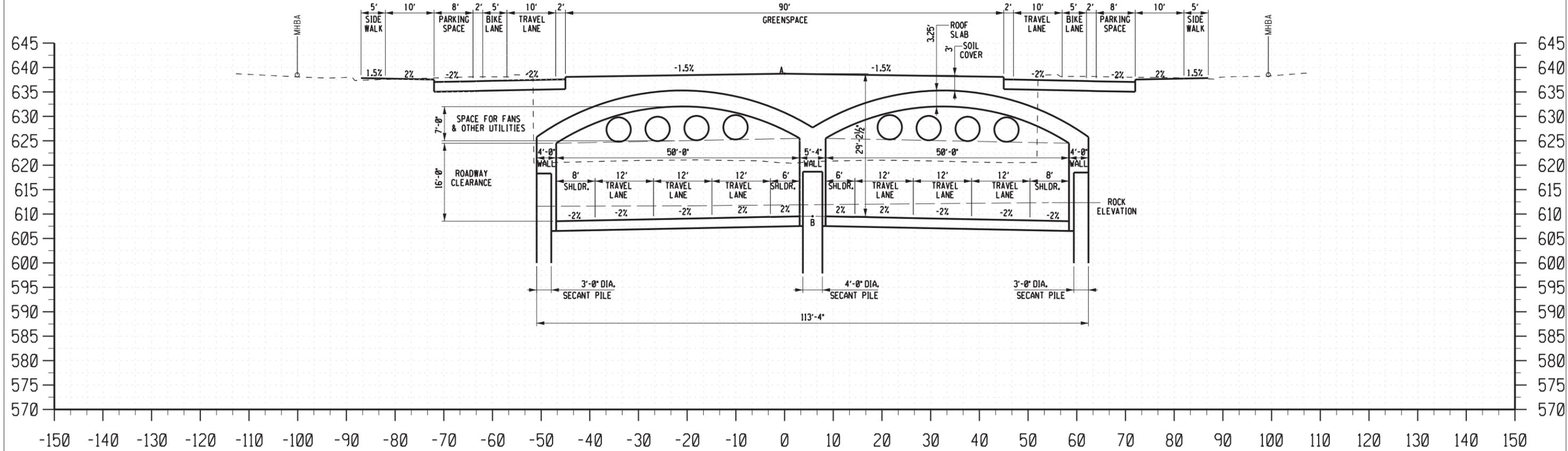
TYPICAL NORMAL SECTION (STA. 98+00 SHOWN) - FLAT ROOF SLAB WITH 3' SECANT PILES
