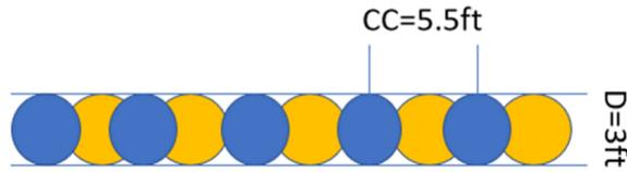
Figure 5 Proposed Secant Pile Configuration (Note: Orange Circles Represent Unreinforced Secant Piles and Blue Circles Represent Reinforced Secant Piles)
