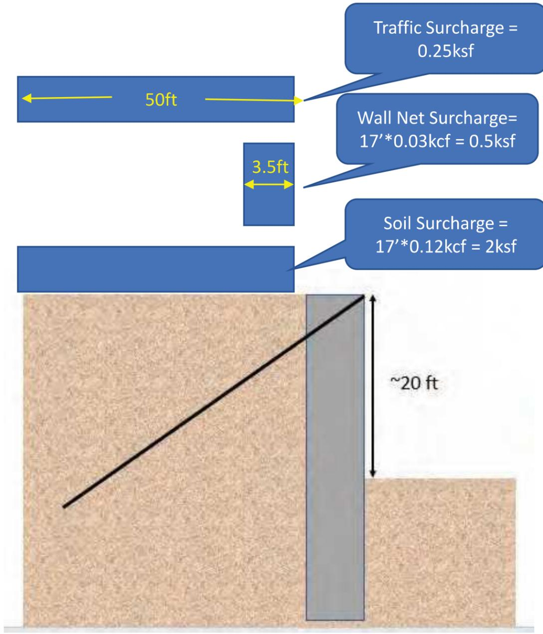
Rock bolt, Drill Hole = 0.5ft, At Top, One Row,
