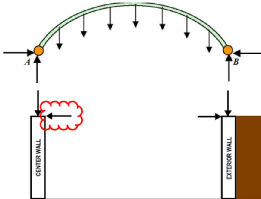
Figure 4 Unbalanced Horizontal Thrust on Center Wall during Construction
