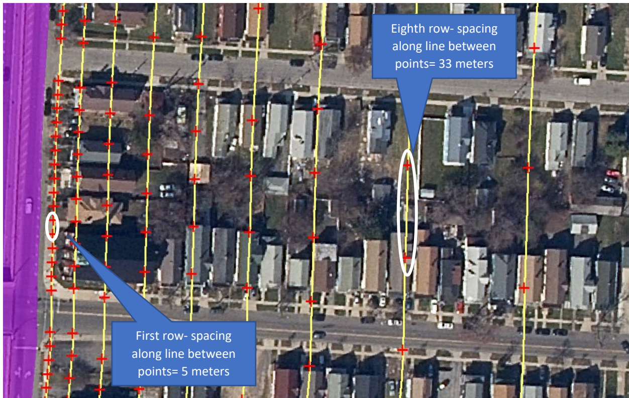
Figure 8: Example of converting lines to points with equidistant spacing along the line
